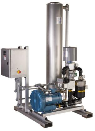
This blower package combines with the FALCO 100 to form an integrated vapor extraction and treatment system. Components are mounted on frames joined by forklift beams. One frame supports the blower, Vapor Control Valve, and accessories. The second frame supports the FALCO 100. This low profile system weighs 595 lb. and is 4' wide, 5' long, and 7' tall. It easily fits in a parking space or a full size pickup truck.
