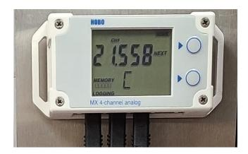
Recorded temperature data supports compliance with regulatory requirements (minimal oxidizer operating temperatures). In addition, temperature data exported to a spreadsheet may be used to estimate VOC concentrations recovered, and cumulative lb/day treated, etc.
