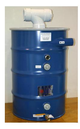
The FALCO Liquid Separator removes liquids and mist from air streams in soil vapor extraction applications. The Separator is installed on the vacuum side of the blower to prevent liquid carryover to the blower and treatment system.
