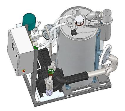
This high flow vapor extraction and treatment system integrates the FALCO 600, SVE Blower, Vapor Control Valve (VCV), and inlet filter onto one stainless steel frame. Assembly weighs 2,270 lbs and is 56" wide, 78" long, and 87" tall. System is fully tested and can be economically shipped by common carrier (flat bed not required).
