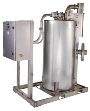
The FALCO 600 electric catalytic oxidizer treats air streams contaminated with volatile organic compounds. The catalyst provides VOC destruction efficiencies up to 99.5%. Operation, including startup, is fully automatic. Controllers accurately regulate input loading and temperatures. The controls adjust a FALCO Vapor Control Valve (VCV) to maintain safe maximum input concentrations. Automatic shutdown results if temperatures exceed limits.
