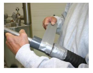
Prepare a shop vacuum with 48" piece of ¾" tubing. Use ¾" Electrical Metallic Tubing (EMT). Duct tape the tubing to the end of the vacuum hose.
