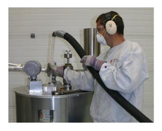
Use the shop vacuum and tubing to vacuum out all the catalyst through the larger (2") Catalyst fill plug. (Caution: Do not bend divider plate). Use a flashlight to inspect the catalyst chamber for damage. Call Falmouth products before proceeding if damage is present.
