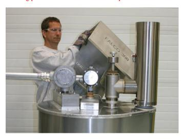
Turn off all power to the FALCO. Lockout/Tagout power supply to the FALCO 300. Remove screws holding FALCO 300 heat shield with a screwdriver. Remove Heat shield.
