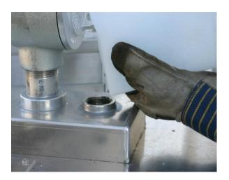
Fill the small port with catalyst. The catalyst must be evenly distributed in the catalyst chamber.
