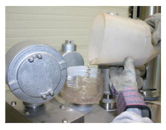
Make a funnel and a scoop out of clean plastic containers. Pour new catalyst into the catalyst chamber through the two fill plugs.
