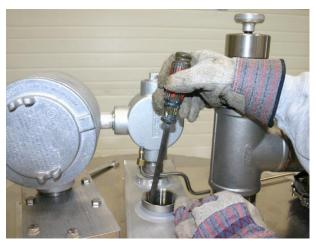
Gently distribute the catalyst with a large clean flat head screwdriver. Continue to fill the chamber until it is within ½" from the top of both fill ports. Screw in the fill plugs. Assembly is the reverse of disassembly. The catalyst level will settle and should be topped off after initial operation. Catalyst level should be checked again after two weeks of operation and topped off as necessary.
