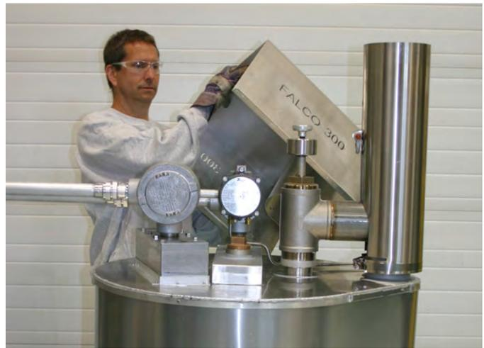
Turn off all power to the FALCO. Lockout/Tagout power supply to the FALCO 300. Remove screws holding FALCO 300 heat shield with a screwdriver. Remove Heat shield.
