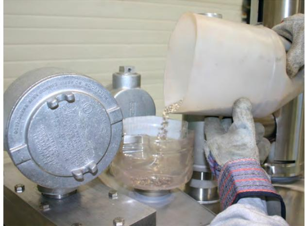
Make a funnel and a scoop out of clean plastic containers. Pour new catalyst into the catalyst chamber through the two fill plugs.
