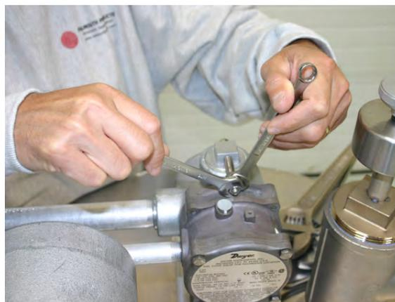
Unbolt the pressure switch with two 7/16” wrenches.
