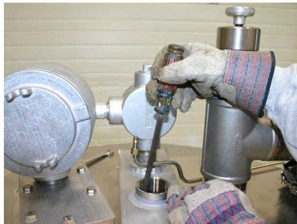
Gently distribute the catalyst with a large clean flat head screwdriver. Continue to fill the chamber until it is within 1/2" from the top of both fill ports. Screw in the fill plugs. Assembly is the reverse of disassembly. The catalyst level will settle and should be topped off after initial operation. Catalyst level should be checked again after two weeks of operation and topped off as necessary.
