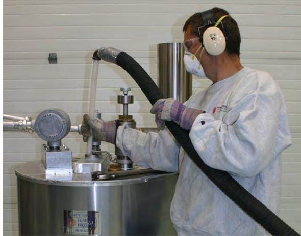
Use the shop vacuum and tubing to vacuum out all the catalyst through the larger (2") Catalyst fill plug. **(Caution: Do not bend divider plate).** Use a flashlight to inspect the catalyst chamber for damage. Call Falmouth products before proceeding if damage is present.
