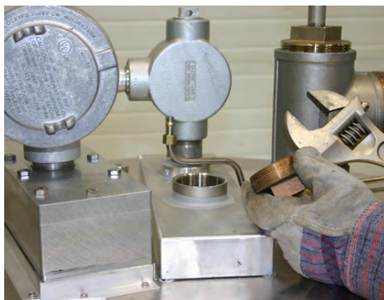
Put on dust mask, safety glasses, and ear protection. Use an adjustable wrench to remove the 2” Catalyst fill plug.
