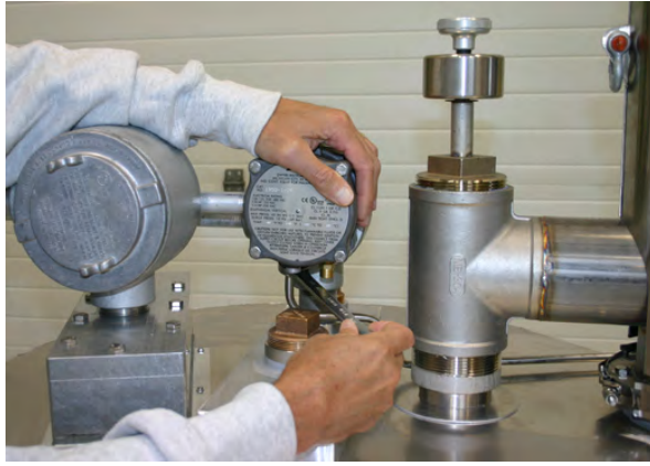
Disconnect the tube from the bottom of the pressure switch (“+” or high pressure port) with a 5/8” wrench.
